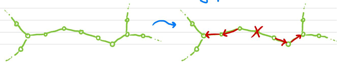
Iterative process: On each step, delete a small number of vertices & orient some edges
